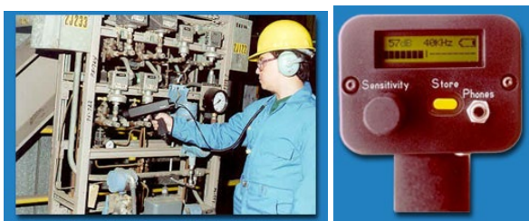
Figure 2 - The Ultraprobe 9000 leak detector
