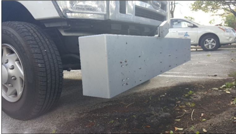
Figure 4. Inertial Roadway Profiler Sensor Bar
