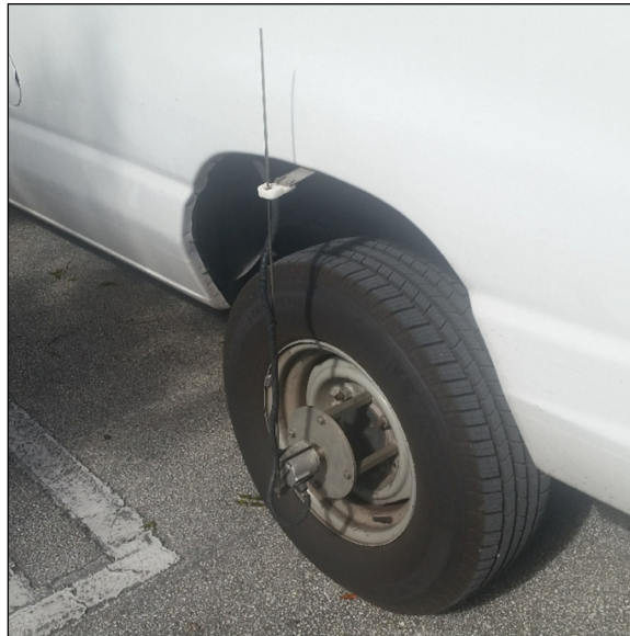
Figure 5. Inertial Profiler Distance Measuring Equipment
