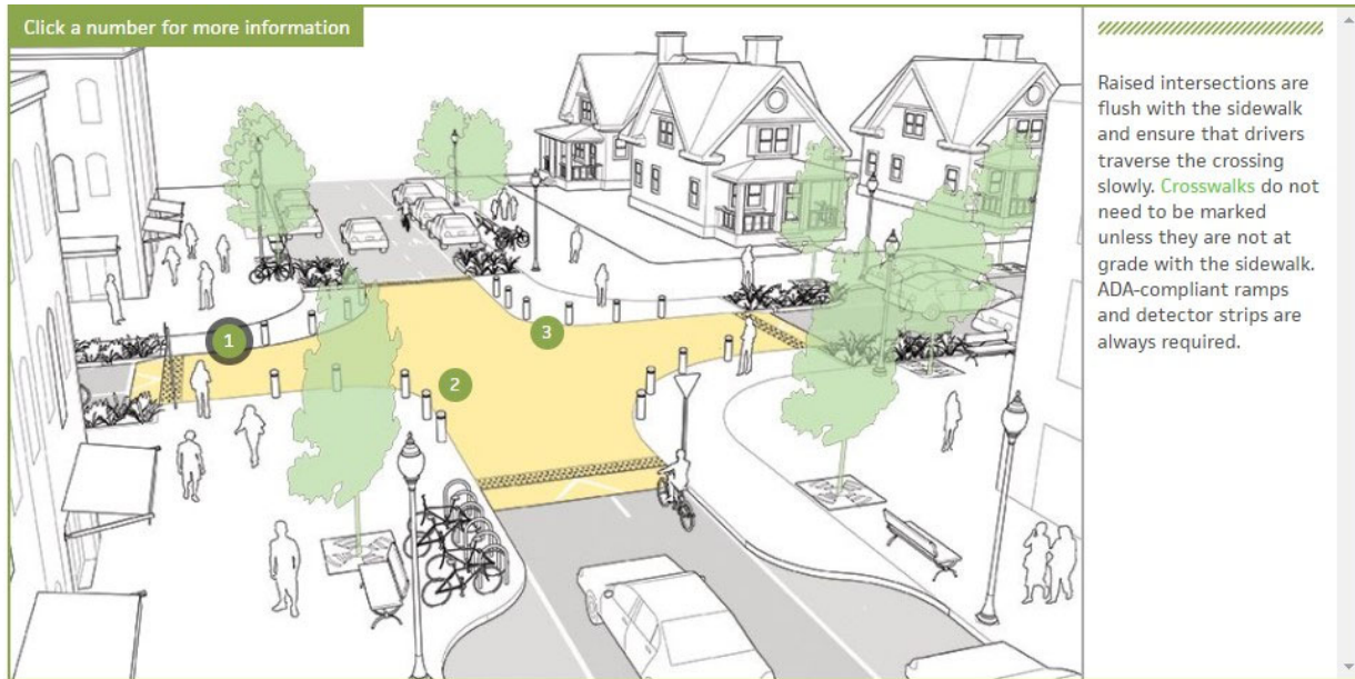
Figure 28 NACTO Raised Intersection
