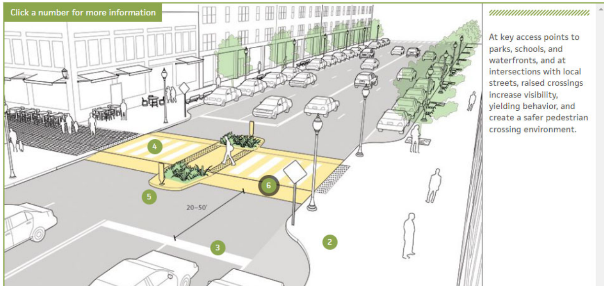
Figure 32 NACTO Raised Speed Table
