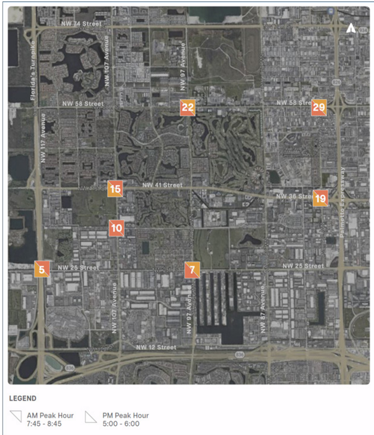
FIGURE 10-5: OVERALL FUTURE 2045 PROJECTED INTERSECTION LEVEL OF SERVICE (LOS)
