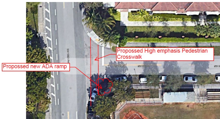
Location 6- NW 88 St and NW 112 Pl: Proposed pedestrian crosswalk. Milling and resurfacing the east-west area.
